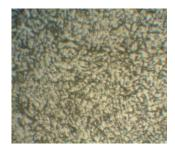
**Figure -7(c):** Microstructure of the HAZ of the butt joint with groove angle x-60°
