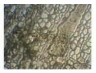
figure -6(c): Microstructure of the weld joint for butt joint with butt angle x-60°
