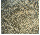
**Figure- 7(b)** :Microstructure of the HAZ of the butt joint with groove angle v-90°
