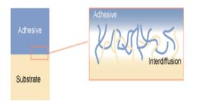
Fig 4.1 Diffusion mechanism
