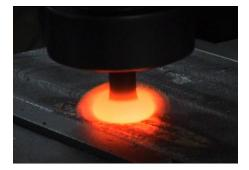
Fig 3.9 a layer of copper coating formed over mild steel
