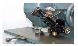
Fig 4.20 Vickers hardness testing machine
