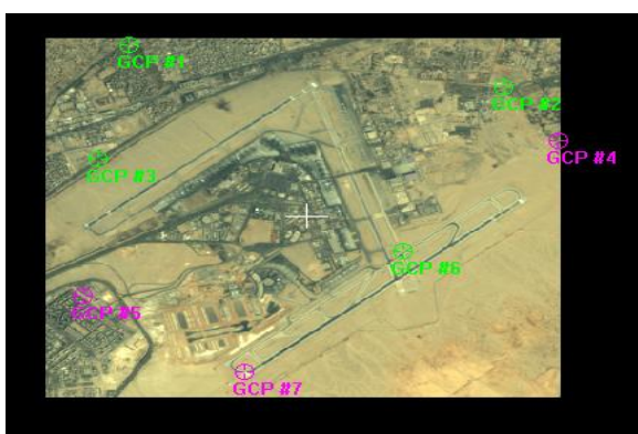
Fig - 5: Distribution of used GCPs [Green Color] and Distribution of CPs [Magenta Color] in case study number (10) for the first scenario that gives the best Total RMS error
