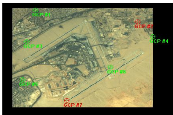
Fig -6: Distribution of used GCPs [Green Color] and Distribution of CPs [Red Color] in case of study number (7) for the second scenario that gives the best TRMS error
