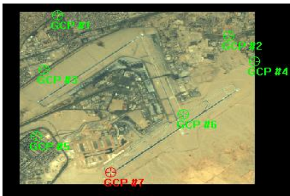
Fig - 7: Distribution of used GCP [Green Color] and Distribution of CPs [Red Color] in case (1) for the third scenario that gives the best Total RMS error
