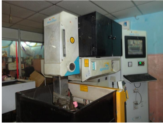
Fig 4 Wire electrical discharge machine
