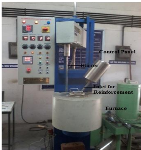
Fig 1 Stir Casting Set up
