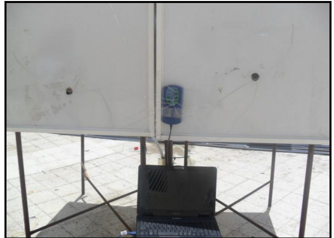
Fig -3: Multi-channel temperature recorder
