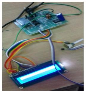
Fig.4: Temperature measurement in slave module
