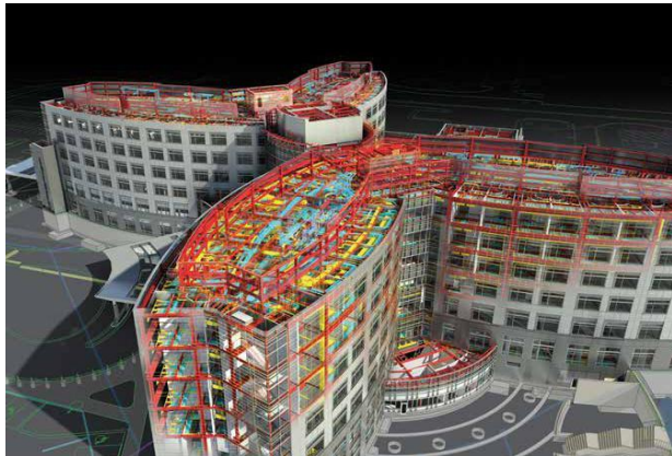
Fig-2 A 3-D model design of a building using BIM.
