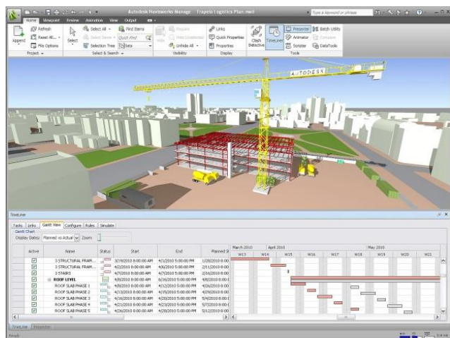
Fig-3 -- Scheduling timeline is collaborated with 3-D Model of Structure taking time as 4 th Dimension
