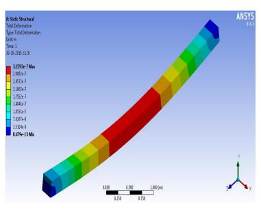
Fig 4 Total Deformation Of A Beam
