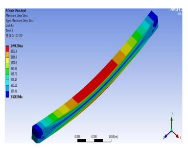
Fig 3 Shear Stress Of A Beam
