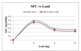
Figure -3: Variation of specific fuel consumption with load
