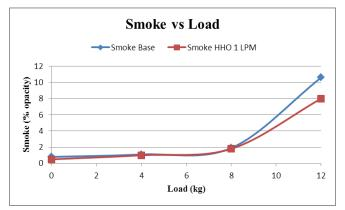
Figure -8: Variation of smoke with load
