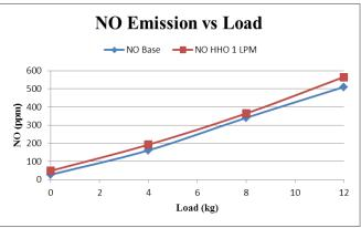
Figure -7: Variation of NO emission with load
