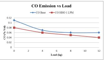
Figure -6: Variation of CO emission with load
