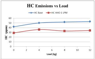
Figure -5: Variation of HC emission with load
