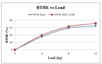
Figure -2: Variation of brake thermal efficiency with load
