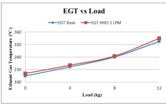
Figure -4: Variation with exhaust gas temperature with load
