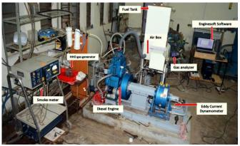
Figure -1: Experimental Setup
