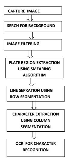
Fig 1. Steps for number plate recognition
