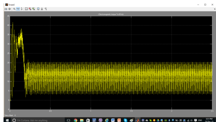
Fig -7: Open Loop electromagnetic torque waveforms
