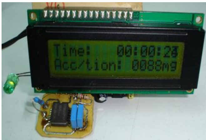
Fig -5: Circuit Diagram of Accelerometer sensor with Microcontroller
