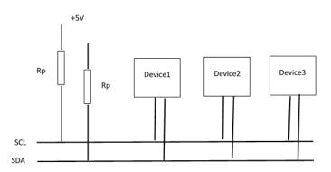
The devices on the I2C bus are either masters or slaves. The master is always the device that drives the SCL clock line. The slaves are the devices that respond to the master.
