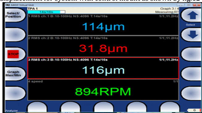
Fig.12: FFT displacement result of system with control mount for 894 rpm.
