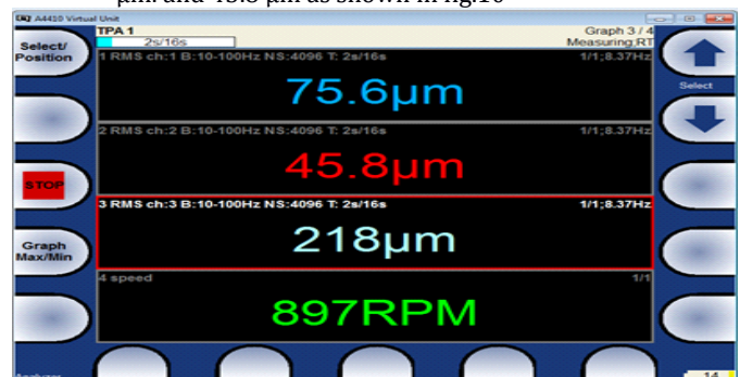
Fig 9: Displacement of system at 897 rpm without control mount
