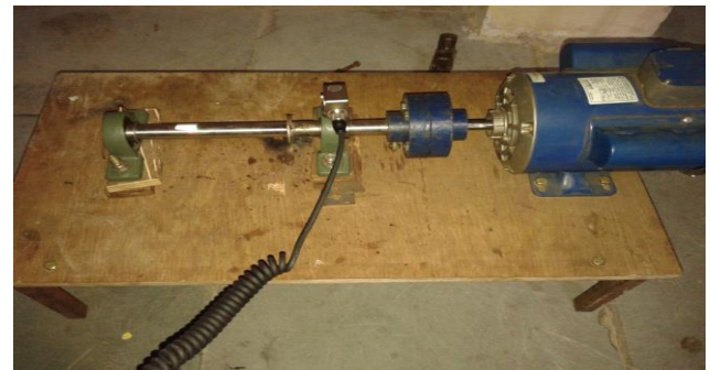
Fig.8 : System without control mount
