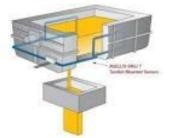
Fig.1.1-Typical Tundish Design
