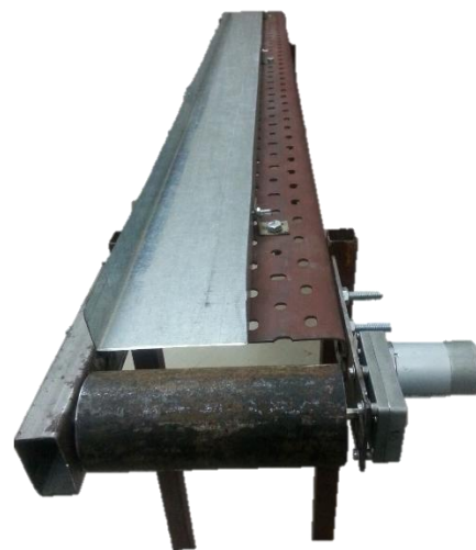
Fig. 6 DC motor connection to the conveyor system
