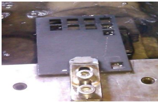
Fig -3: Actual Cutting of Graphite Plate by WEDM
