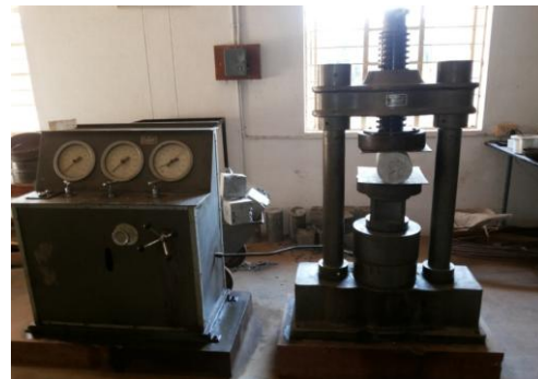
Figure 6.3 compressive strength testing machine with cylinder specimen
