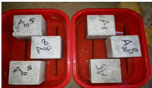
Figure 6.4 concrete specimen applying paraffin wax for sorptivity
