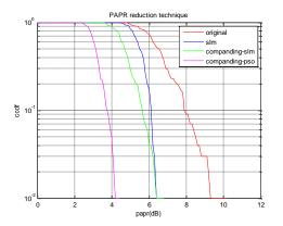
Figure3: Standard CCDF v/s PAPR calculation graph with QAM 16
