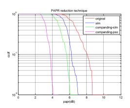
Figure 2: Standard CCDF v/s PAPR calculation graph with QPSK
