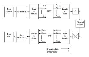
Figure 1: Basic block diagram of OFDM transceiver [35]
