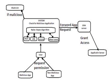
Fig. 2. Architectural Diagram of Proposed System
