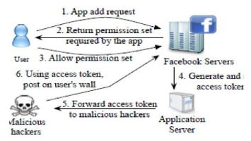
Fig. 1. Architectural Diagram of Existing System.
