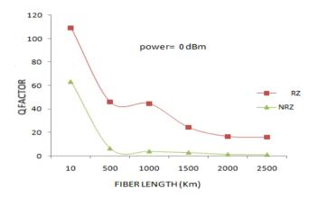
Fig 3 Q factor v/s fiber length (power=0dBm)
