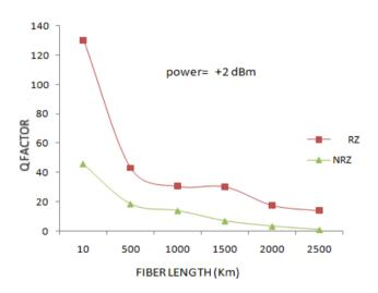
Fig 4 Q factor v/s fiber length (power= 2dBm)
