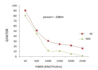
Fig 2 Q factor v/s fiber length (power= -2dBm)
