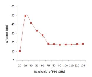
Fig 5 Q factor v/s Bandwidth (GHz)
