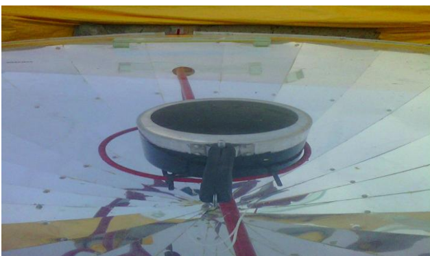
Figure 4: Receiver surface with black coating
