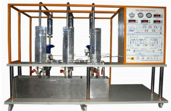
Fig-1: Physical setup of three tank interacting system
