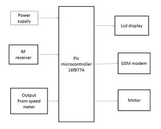
Fig. 2. Receiver block diagram.
