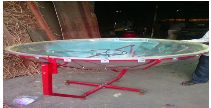
Figure 2: System Details for Steam generation device with glass cover
