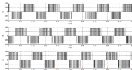
Fig-16: Voltage Output of SPWM
