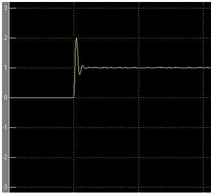
Fig.4.1 Response of maglev system with classical PID design
