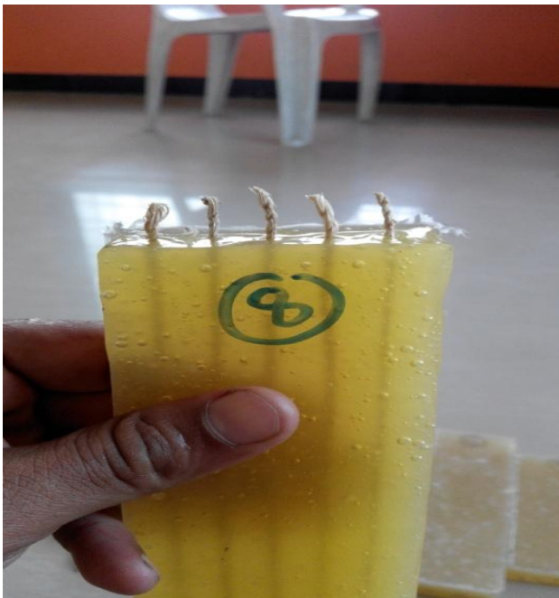
Double laminated Specimens
