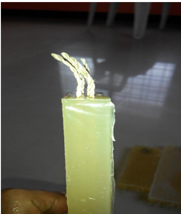
Double laminated Specimens
