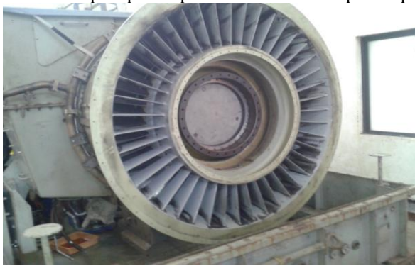
Fig.1.2. Air compressor inlet
