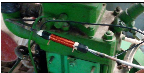
Fig-7: Installation position of solenoid magnetic coil
