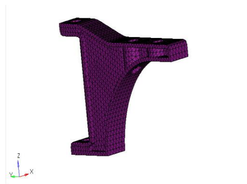
FIG-2 Meshed model of fuel tank bracket
