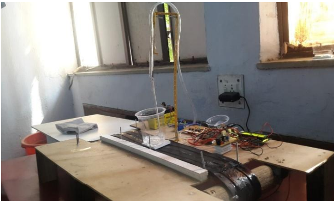
Fig- 7: Flat belt conveyor
