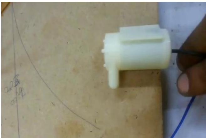
Fig- 8: Rotary motor and pump mechanism
