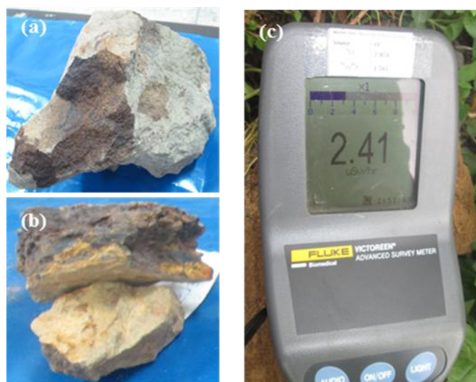
Figure 1. Photographs of two categories of stones (a and b) collected from different locations of Bangladesh; (c) A survey meter reading of a stone of category (a).
