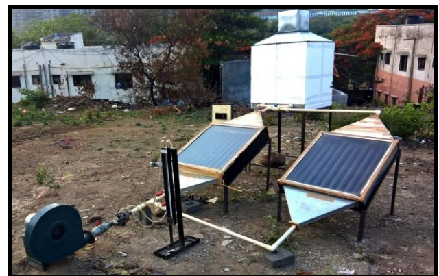
Overall view of solar dryer (Side View)
