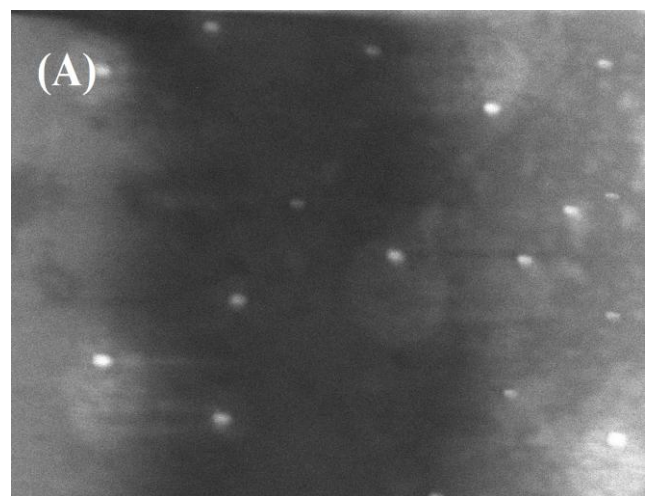
Figure 11: SEM images of APTMS Au@Ag core-shell thin film nanoislands (A) before and (B) after ozonation.
