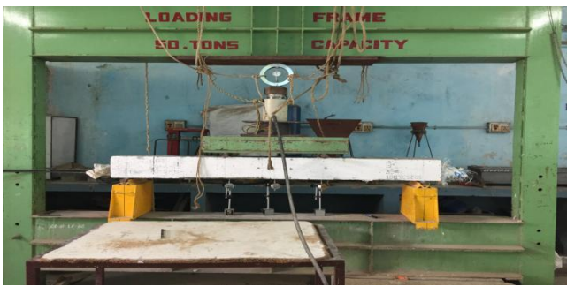
FIG 4: Test set up on loading frame
