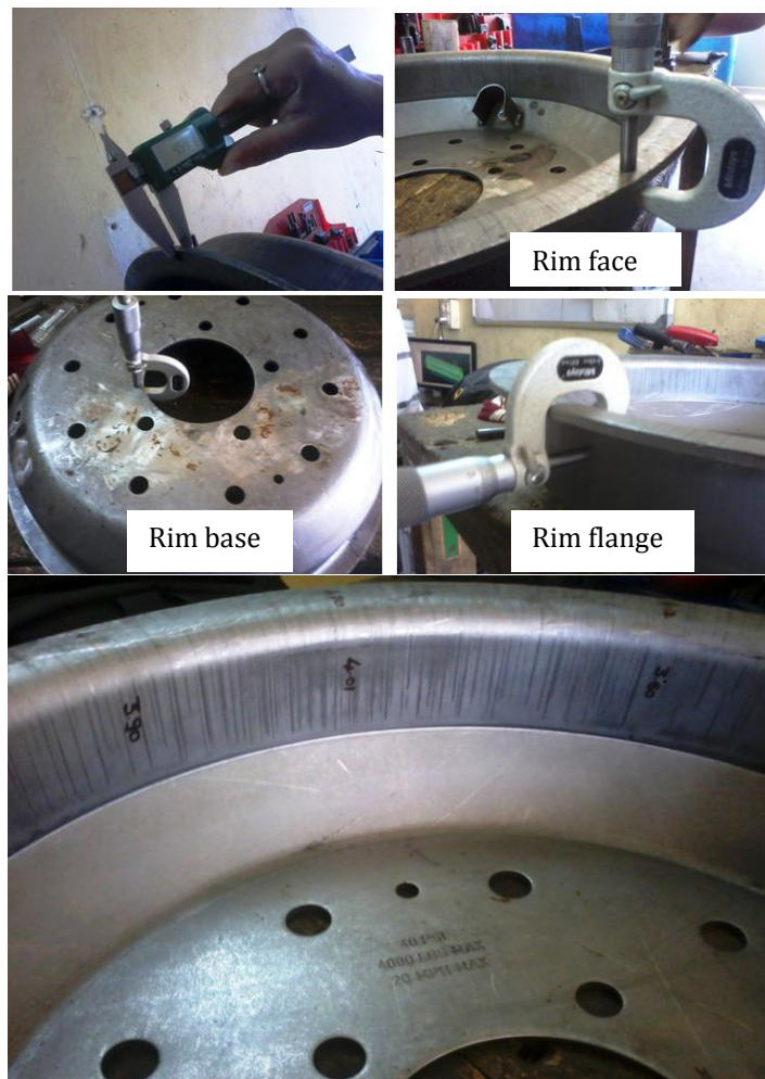
Fig-16: Thickness measurement of the drawn rim
