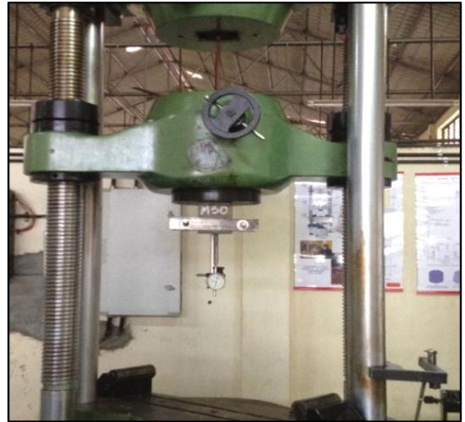
Fig -1: Pull Out Test Setup
