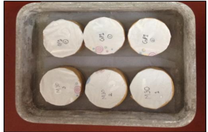
Fig -2: Sorptivity test set up
