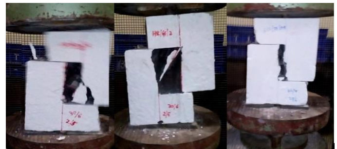
Figure 3(b): Failure pattern in Glass fibres reinforced push-off specimens
