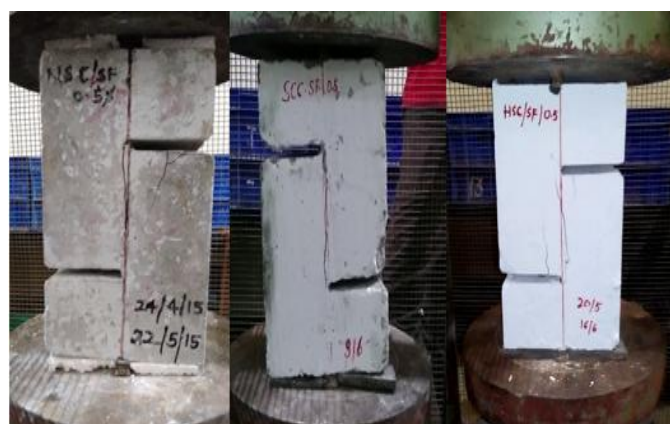
Figure 3(a): Failure pattern in Steel fibres reinforced push-off specimens
