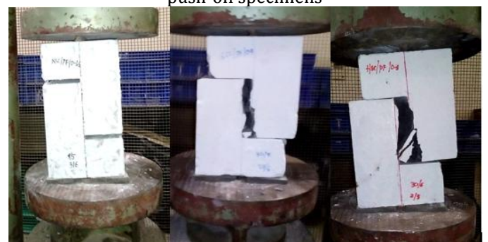
Figure 3(c) Failure pattern in Polypropylene fibres reinforced push-off specimens
