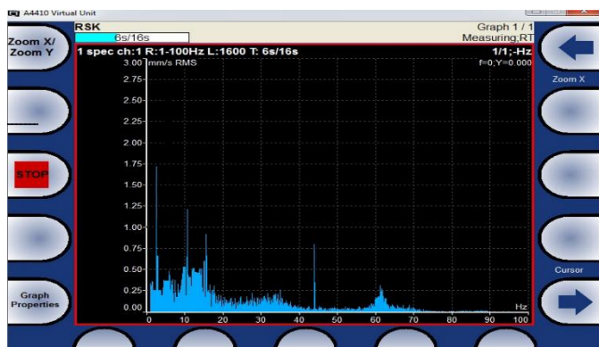
Fig - 15: Frequency Response for 26 ft Blade.
