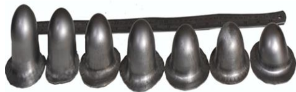
Figure-15: the appropriate produced piece using hydromechanical deep drawing process
