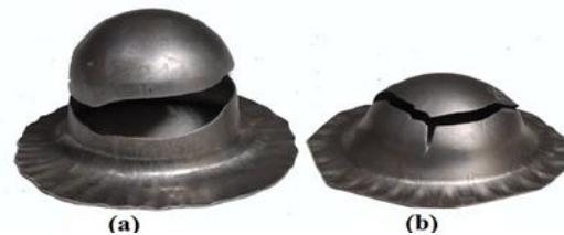
Figure-14: tearing sample a) traditional deep draw b) hydromechanical deep draw
