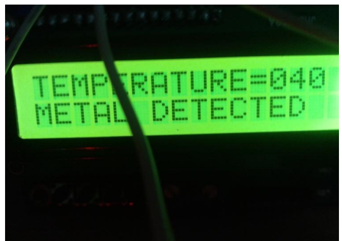
Figure 5: Temperature measured and metal object detected
