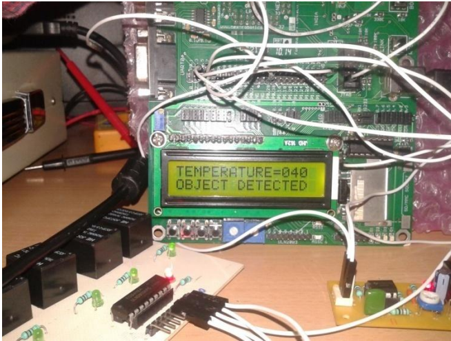
Figure 6: Temperature measured and object detected by IR Sensor
