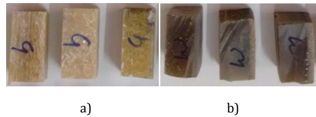
Fig-3: Compression test specimens of a) Epoxy b) Epoxy and Walnut shell powder
