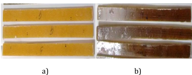
Fig-1: Tensile test specimens of a) Epoxy b) Epoxy and Walnut shell powder
