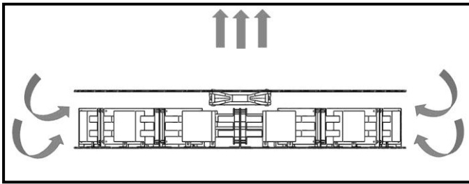
Fig-7 Airflow within the Power Conversion Unit
