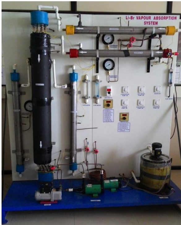
Fig-3: Assembly of Experimental set up for LiBr-H 2 O absorption system
