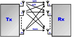
Fig-2 General outline of MIMO system antenna
