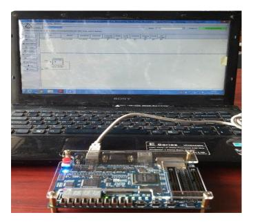
Fig -3: Hardware setup for TRNG.
