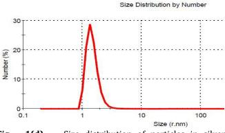
**Fig – 1(d):** Size distribution of particles in silver nanofluid after one week
