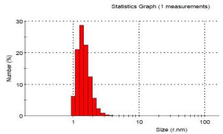
**Fig – 1(c)** Size distribution of particles in silver nanofluid after one week
