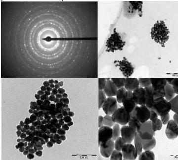
**Fig – 3:** (a) diffraction pattern, (b) 500nm, (c) 200nm, (d) 50nm: TEM images of silver Nanofluid
