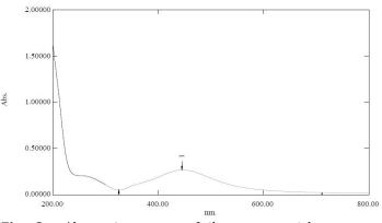
Fig - 2: Absorption spectra of silver nanoparticles.
