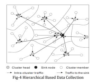
LEACH (Low Energy Adaptive Clustering Hierarchy) is first clustering protocol which gave the clustering concept by randomly selecting the cluster head. It operates into two phase, set up phase and steady state phase. LEACH suffered from following drawbacks:
