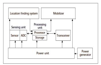
Fig-2 Components of Sensor Node [2]
