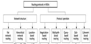
Fig-3 Classification of routing protocols
