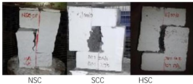
NSC SCC HSC Figure 3: Failure pattern in push-off concrete specimens
